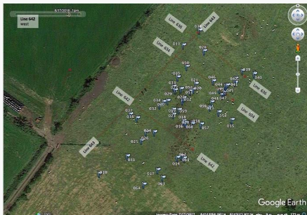
Plotting the survey data, the GPR and metal detector hits at Bentra. Image by Alastair Ruffell
